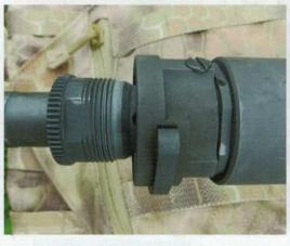
prong flash-hider to my E category BCM AR15 and headed to the range to re-zero and check the points of impact with the ASE both fitted and removed. This check is important if you plan on firing your rifle suppressed and unsuppressed, because the point of impact will move when a significant weight (the suppressor) is fitted to the end of your rifle.
