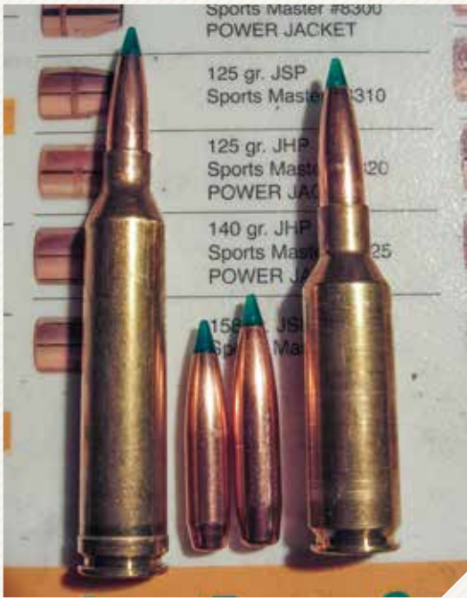
⬆ A view of the .264 Win Mag (left) and 7mm SAUM cartridges and projectiles.
